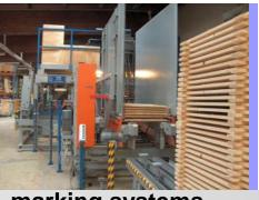
Not only the product specification but also client demands are considered for the design of the stacker. The best machine according to the client demands is our goal. The machine can be set up complete automatically.
